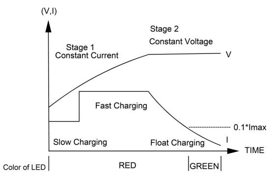
Note: This charging curve is for Li-Ion battery.
